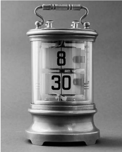
Fig. 1.3 A clockwork digital clock
